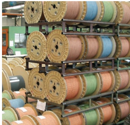
500mm \varnothing process ABS reels. The product is single core for telecommunication cable
