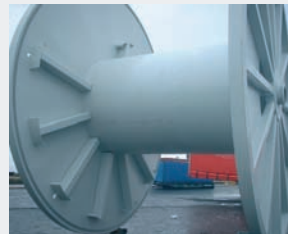
6.1m \phi shipping drum with a skeletal ramp, designed for a load of 115 tonnes
