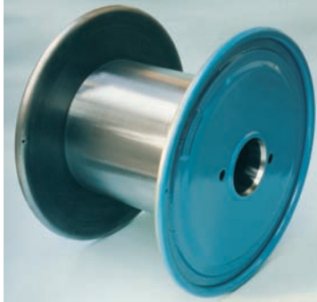
BP 630 \phi with 127mm bore to Din 46397 dynamically balanced ISO 1940, G16
