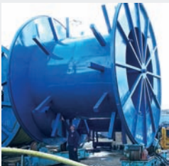
Offshore transportation drums 6.0m \phi for a load of 50 tonnes
