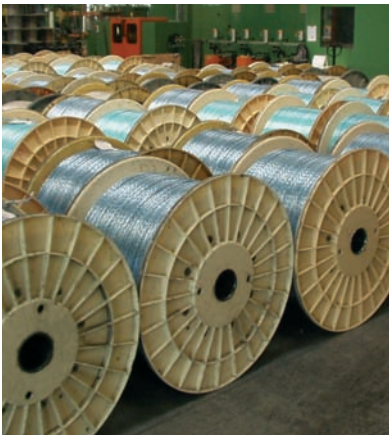
1000mm \varnothing process ABS reels, seen at the end of the stranding line. The product is data telecommunication cable
