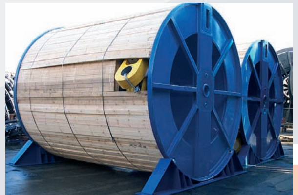
4.6m \phi offshore transportation drums, on offshore cradles, designed to carry 110 tonnes
