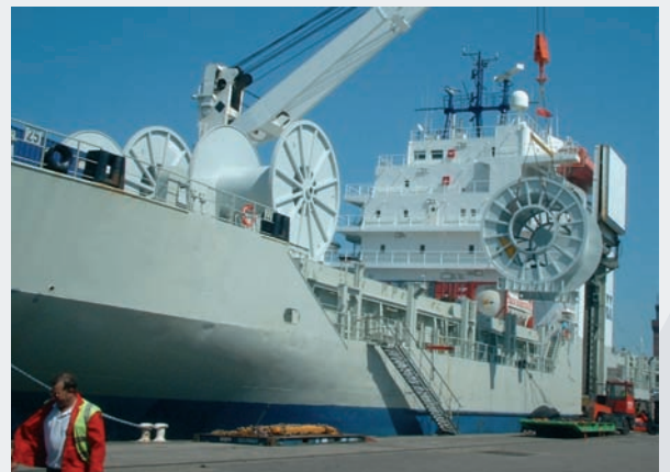
The 5.5m \phi shipping drum being lifted is intended for use with the Coflexip Drive System. All 3 shipping drums are designed for umbilical cables in offshore applications
