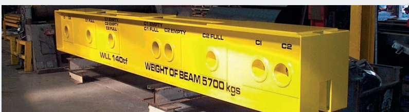
Offshore lifting beam designed with a SWL of 140 tonnes
