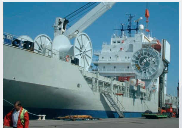
The 5.5m ø shipping drum being lifted is intended for use with the Coflexip Drive System. All 3 shipping drums are designed for umbilical cables in offshore applications
