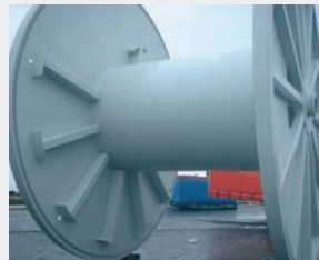
6.1m ø shipping drum with a skeletal ramp, designed for a load of 115 tonnes
